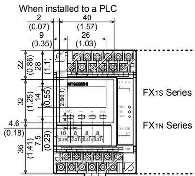
Note: These dimensions measured from the left side are common to the FX1S and FX1N Series.
